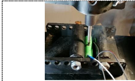
Figure 2. Experiment stand for 18650 cell.
